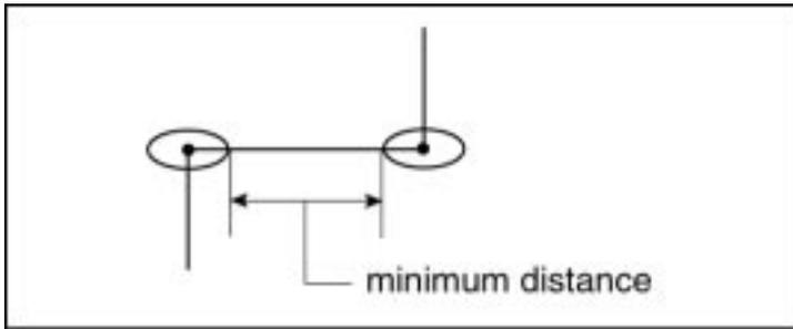
The **buried\_via\_gap** is the gap between coincident vias for hybrid circuits. The following rules apply:
