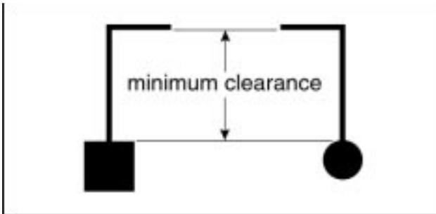
The **smd\_to\_turn\_gap** clearance is defined as the minimum clearance from any SMD pad to the first 90 degree turn in the wire.
