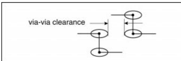
If a **buried\_via\_gap** is used, this value defines the clearance between buried vias that do not share a common layer, as shown in the following figure. The **layer\_depth** option specifies the number of layers over which the clearance rule applies. See also the **bbv\_ctr2ctr** setting in the [<control\\_descriptor>](#).
