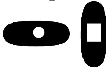
**Circle.** To define a solid aperture, enter only the diameter. To define a hole, enter one dimension for a round hole, two for a rectangle. The hole must fit within the aperture. For a square hole, X must equal Y. Both aperture and hole will be centered. For example,
