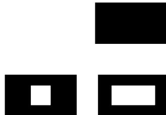
**O,**      **<X-axis dimension>X<Y-axis dimension>[X<X-axis hole dimension>[X<Y-axis hole dimension>]]**
