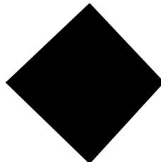
**Regular polygon.** May be solid or open. To define a solid aperture, enter only the outside dimension and number of sides (3 to 12). The first point is located on the X axis. May be rotated  $\pm 360^\circ$  from the X-axis. If open, the hole must fit within the outside dimension. *Note: If you use the hole dimension modifiers, you must enter a rotation (even if it is 0).* For example,
