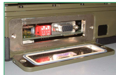
Connectors on the LT450F are directly mounted to the case. The battery clip can also be seen here (right)
