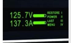
The Model 2001's multiple display capability makes it easy to gather several pieces of information simultaneously from different aspects of a single signal. One of these displays is ideal for power supply monitoring because it shows the DC voltage of the supply's output, the AC noise level, and the frequency of that noise all at once, which simplifies tracking down the source of the noise and correcting it.
