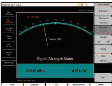
Using the Signal Strength Meter makes locating an interfering signal easy.
