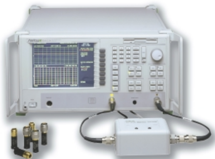
Easy 2-port calibrations using AutoCal®.
