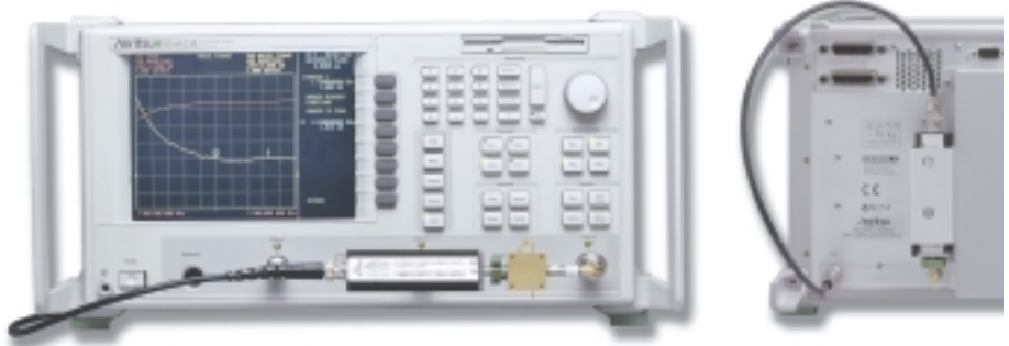
External and internal connections for the Noise Figure measurements choices using Scorpion.
