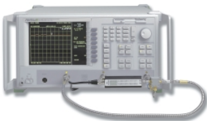
An example of an external Noise Figure measurement on a mixer. With 2 internal sources, Scorpion can provide both the RF and the LO signals to the mixer.
