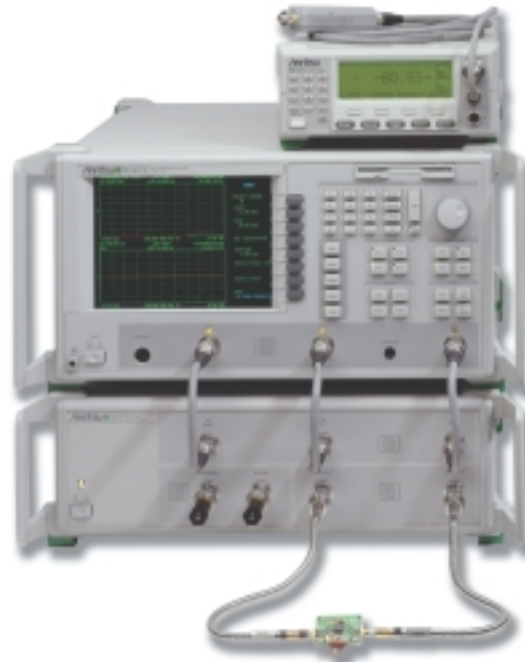
The complete test setup for power amplifier measurements with a single connection.
