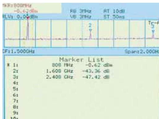
Multi-marker (harmonics measurement)
