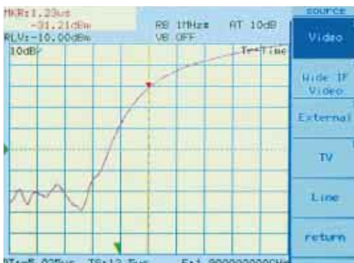
High-speed time-domain measurement (TS = 12.5 \mu s)
