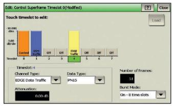
Use the Model 2900-GSM option's waveform edit menu to select the channel type and data type for each time slot.
