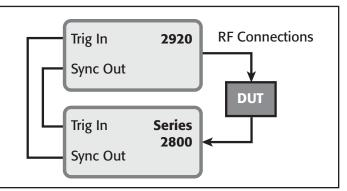
The Model 2920's trigger input and sync output connections simplify synchronizing its operation with that other test instruments, such as Keithley Series 2800 RF Signal Analyzers, in high speed measurement applications.
