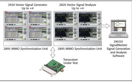
This 4×4 MIMO test system ensures precise synchronization and low jitter when testing WiFi, WiMAX, and other MIMO devices and equipment.
