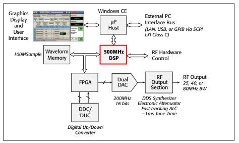
The key components of the Model 2920's DSP-based software-defined radio architecture are optimized for high accuracy and fast test throughput while reducing instrument cost and rack space requirements.
