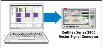
Create waveform files off-line on a PC with Keithley's free SignalMeister waveform creation software, then download them to the ARB memory of any Keithley Series 2900 RF Vector Signal Generator.
