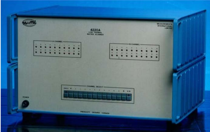
**Automated Low Thermal Matrix Scanner - 20 Channel 30 Amp**
