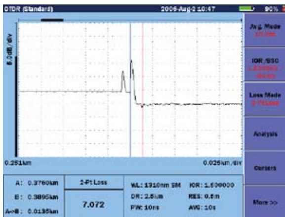
Fig. 1: With its high resolution optics, the MT9083A provides exceptional detail allowing users to quickly determine where the problem is-even when events are closely spaced.
