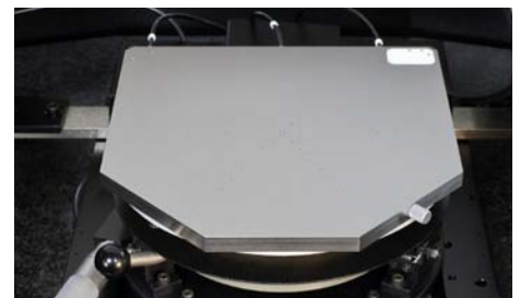
Figure 4. Dedicated RF chuck with excellent surface planarity and small vacuum holes
