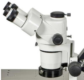
Figure 20. Trinocular 6.7x stereo zoom microscope with 20x eyepieces included in EPS200RF package
