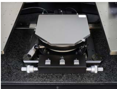
Figure 19. Chuck stage design with integrated coarse X/Y movement, fine X/Y positioning and fine-theta adjustment
