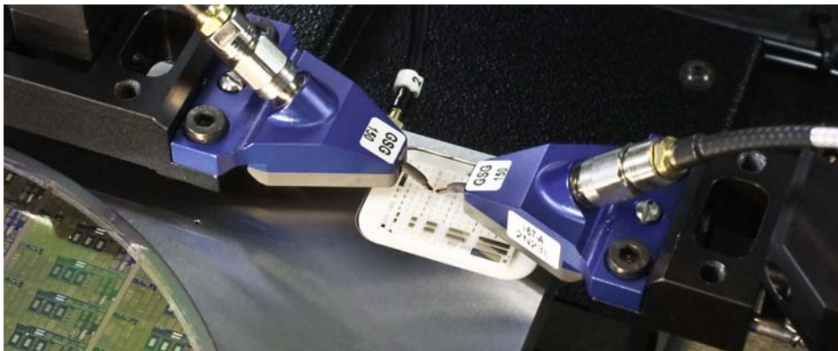
Figure 7. Embedded ceramic AUX chuck for optimized calibration boundary conditions
